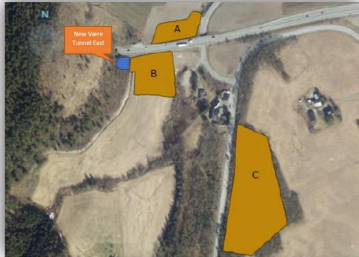
Figure 2. Areas A and B to be filled mainly with tunnels excavation material
