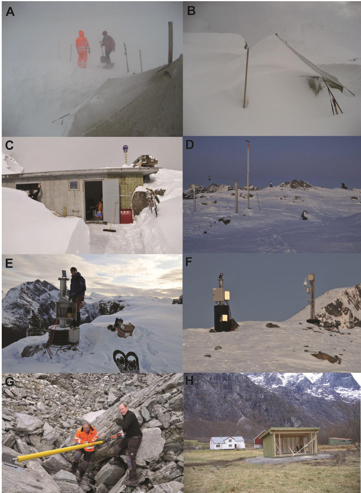
FIGURE 3. PHOTOS FROM ESTABLISHMENT OF DIFFERENT MONITORING ON MANNEN IN 2009. A) AND B) SNOW STORM AND THE TENT CAMP IN OCTOBER; C) BUNKER; D) METEOROLOGICAL STATION; E) ESTABLISHMENT OF LASER SYSTEM LASER SYSTEM; F) LASER TO THE LEFT AND COMMUNICATION ANTENNA AND WEB CAMERA TO THE RIGHT; G) EXTENSOMETER; H) BUILDING FOR THE GROUND-BASED RADAR IN ROMSDALEN.
