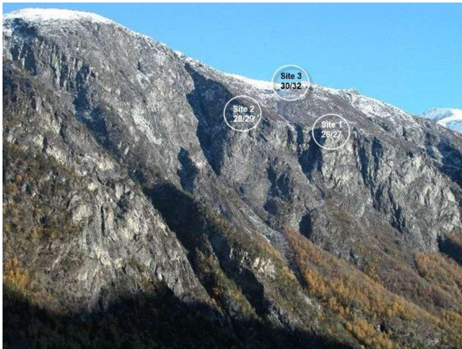
FIGURE 11: PHOTO SHOWING THE LOCATION OF THE RADAR REFLECTOR SITES. SITE 2 CORRESPONDS TO UPPER INSTABILITY AND SITE 1 TO LOWER INSTABILITY.
