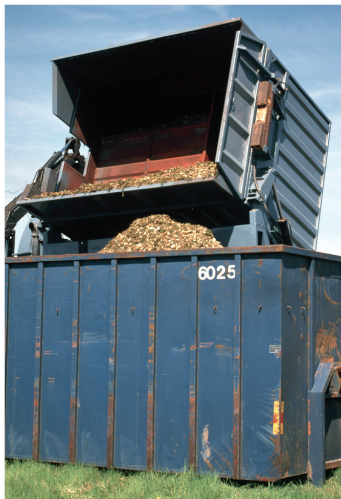
Flis lastes over i container for videre transport (NoBio)
