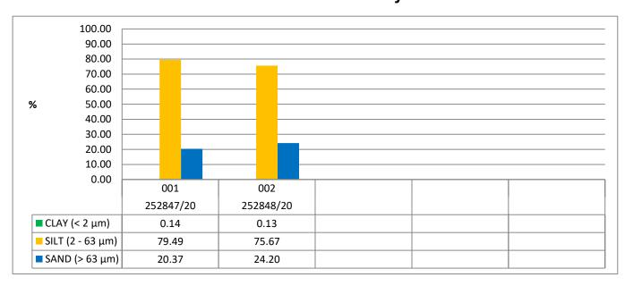
Test method specification: CZ\_SOP\_D06\_07\_120 Grain size analysis using the wet sieve analysis using laser diffraction (fraction from 2  $\mu$ m to 63 mm) Fraction > 0.063 mm determined by wet sieving method, other fractions determined from the fraction "< 0.063 mm" by laser particle size analyzer using liquid dispersion mode. Fractions "Sand >63  $\mu$ m", "Silt 2-63  $\mu$ m" and "Clay <2  $\mu$ m" evaluated from measured data.
