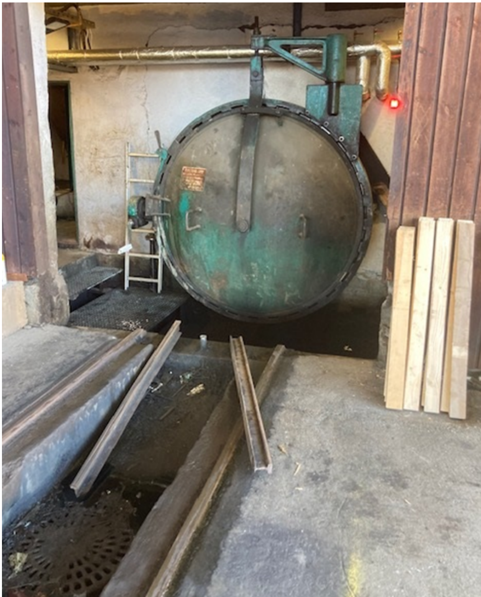
Figur 12: Autoklave for kobberimpregnering
